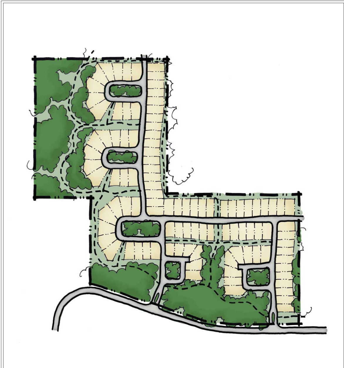
Figure 3.7: Loop and Grid Hybrid Street Network
