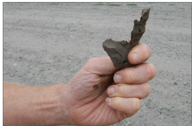
Figure 2. Estimating soil texture by hand (pictured sample is rich in clay). Photo by Andy Bary, WSU
