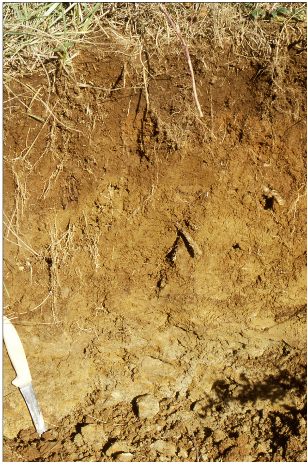
Figure 6. The gray color with mottles in the lower part of this soil profile indicates a seasonal high water table. Photo by Craig Cogger, WSU
