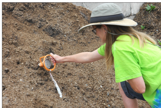
Figure 13. Measuring the temperature of a hot compost pile. Photo by Craig Cogger, WSU
